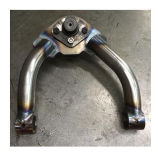
• It's necessary to remove a small amount of material from the "humps" of the factory cross shaft so it will fit inside the new control arm. This can be done with a hand sander until the shaft will pass through the arm.
